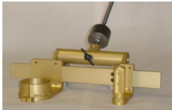
11. Select the hole on the riser that best fits your project. The second hole from the bottom will put your cutter about 3 inches from the base. Each hole is 1 inch apart. Now reinstall the “X” Axis rod.
