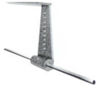
5. With both "Y" axis rods in position on the support angles, slide the Bridge Assembly forward and back several times through its full range of travel. This will help the support angles find their natural position on the base.
