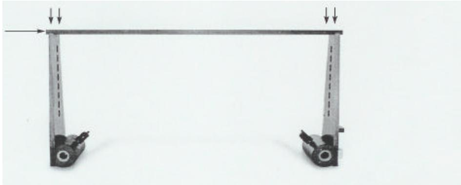
2. Insert the "X" Axis Rod between the bottom holes of the Bridge Uprights. Install a 1" shoulder screw at each end of this rod. (**Model 520,1020, & 1520**) For Model 510,1010, & 1510 slide the "X" Axis rod through the holes and use 3/8-16 button head screws at each end.
