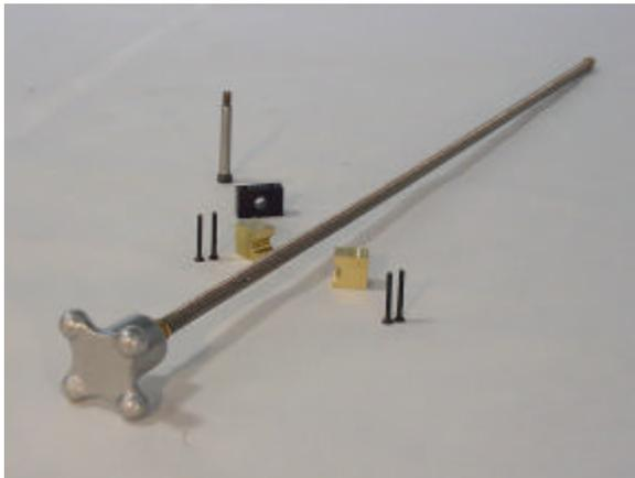
6. The lead screw can be installed on either the left or right or both sides of the Y-axis.
